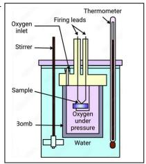
ii. A pure, 0.04600 gram sample of ethanol was burnt in this calorimeter with excess oxygen to raise the temperature of the water by 9.40 °C.
